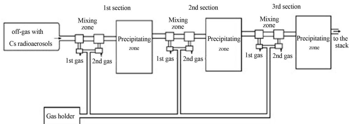
**Figure 1.** New decontamination set-up.
