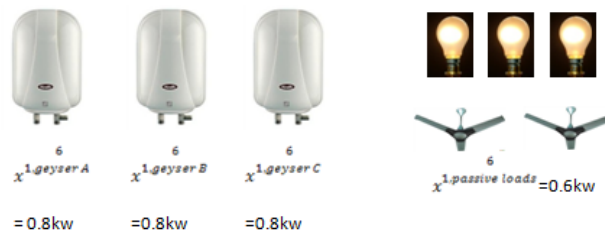
Figure 5. Loads that fall under the blackout region.
