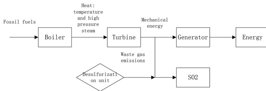
**Figure 3.** Sulfur dioxide emission principle.
