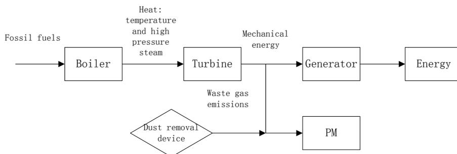
**Figure 5.** The respirable particulate matter emission principle.
