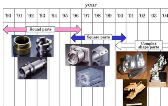
Figure 2. Evolution of parts machined by turning machines (after T. Moriwaki [1]).
