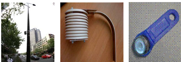
Figure 3. Sensors were installed on lampposts at a height of 3 to 5 meters due to security concerns and local authority restrictions (left). The radiation shield (centre) and the iButton sensor with the miniature data logger that are positioned inside the radiation shield (right). Central Image Source: [23].
