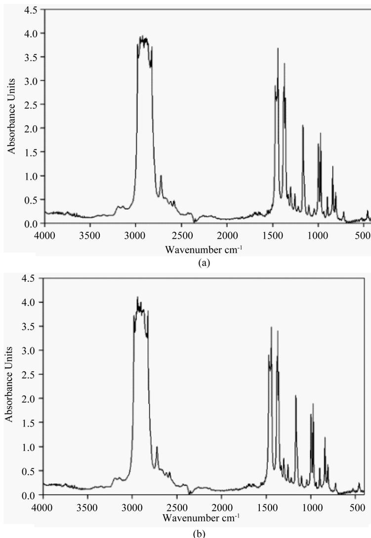
**Figure 10.** FT-IR spectra of Ar/air plasma untreated (a) and 30 s treated (b) BOPP films.
