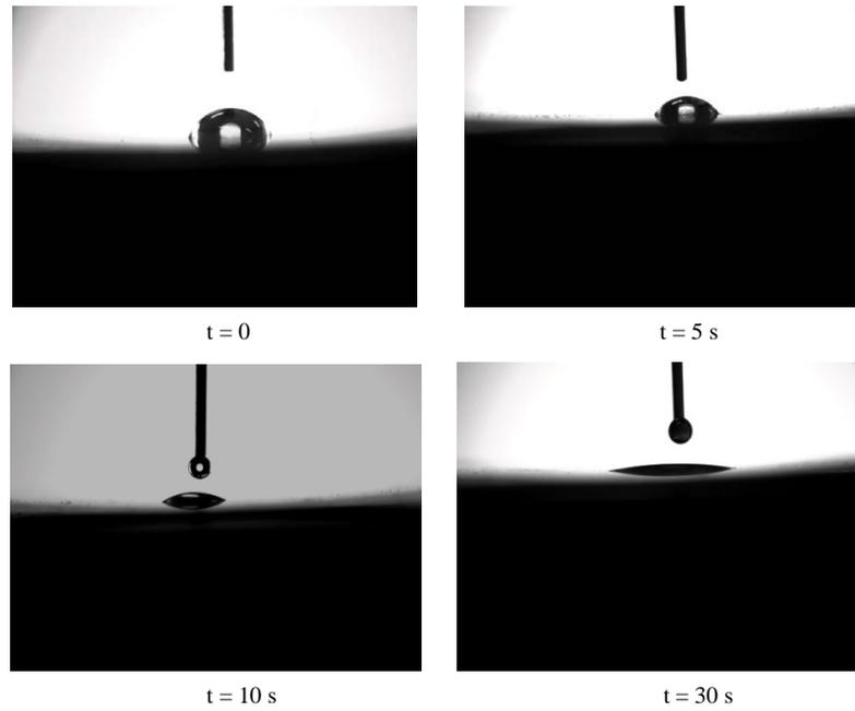
**Figure 4.** The photos demonstrate the relationship between the water contact angle and glow discharge time.
