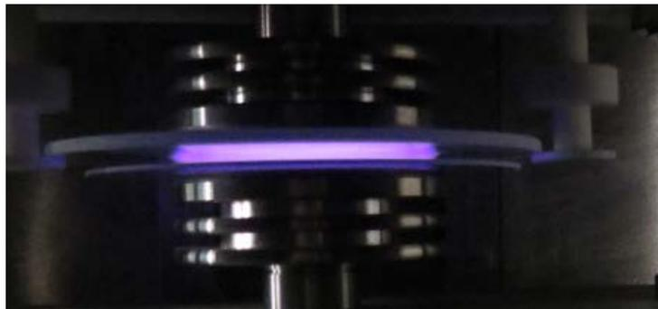
**Figure 2.** A snapshot of glow discharge pattern.
