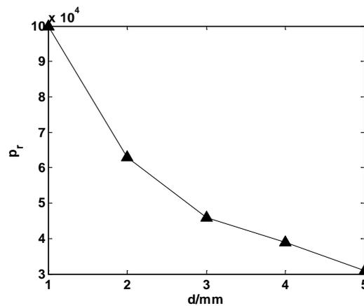
**Figure 5.** Dependence of the maximum pressure  $p_r$  for glow discharge with different discharge gaps  $d$ .
