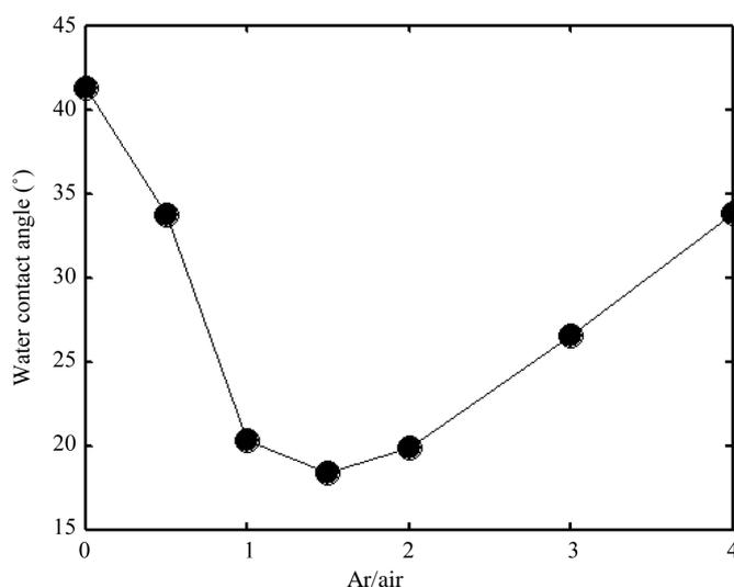
**Figure 9.** Changes of water contact angle with the ratio of Ar/air.
