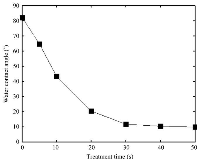
**Figure 7.** Changes of water contact angle with plasma treatment time.
