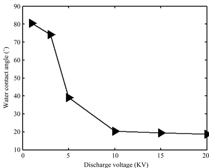
**Figure 8.** Changes of water contact angle with discharge voltage.
