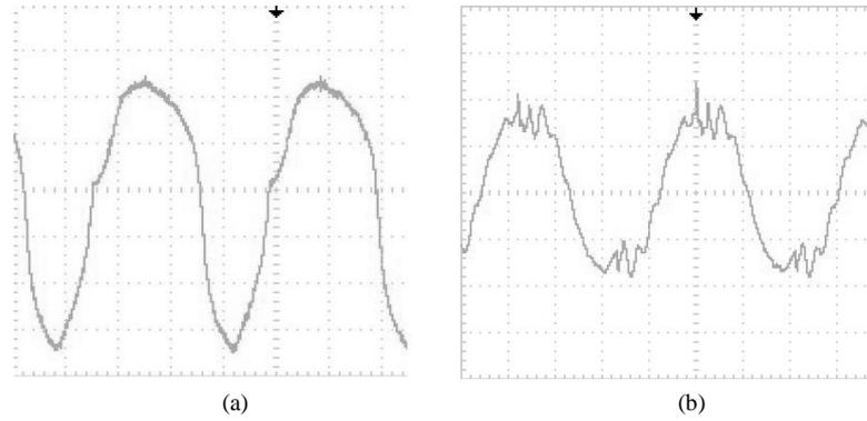
**Figure 3.** Voltage (a) and current (b) waveforms of glow discharge.
