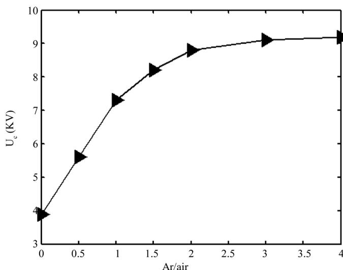
**Figure 6.** Dependence of the minimum glow discharge voltage versus the mixture ratio of Ar/air.
