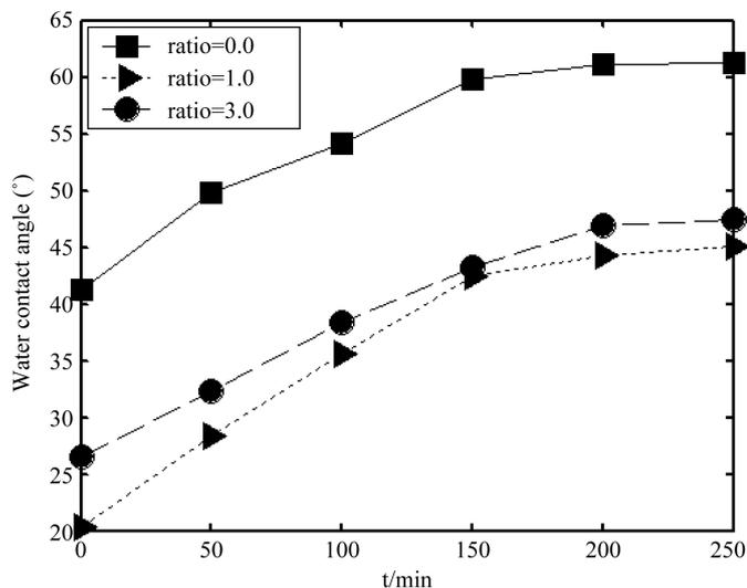
**Figure 11.** Time evolution of the water-contact angle of the modified BOPP membranes in storage in air.
