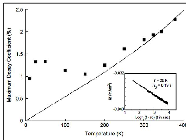
**Figure 4.** The maximum decay coefficient as a function of temperature for the particulate iron in a recording tape media. The dotted line is a plot of the decay assuming classical statistics and using measured values of the parameters. The inset shows a typical measurement ( $M$  vs.  $T$ ) of the decay coefficient.
