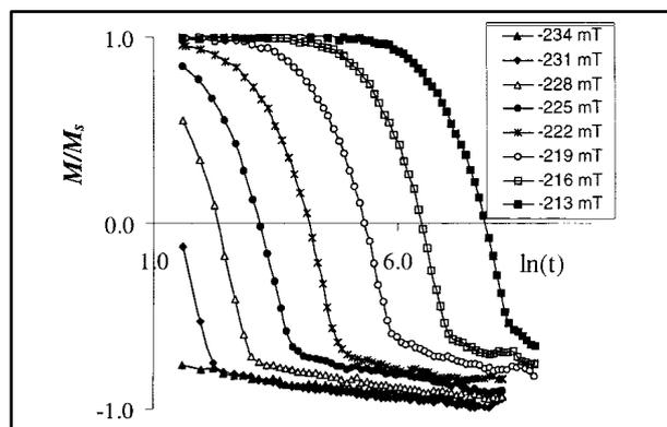
**Figure 5.** Measured aftereffect curves in a (3 Co/10 Pt)<sub>15</sub> multi-layer film.
