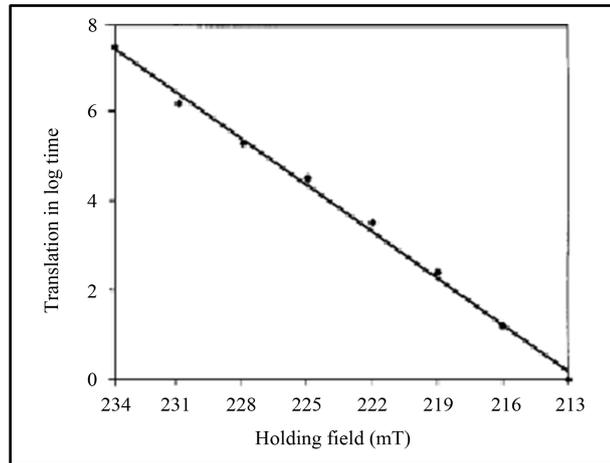
**Figure 6.** The translation, in log time, versus the holding field, in mT, from the CoPt nanopillar data of **Figure 5**. The solid line is a linear regression of the data.
