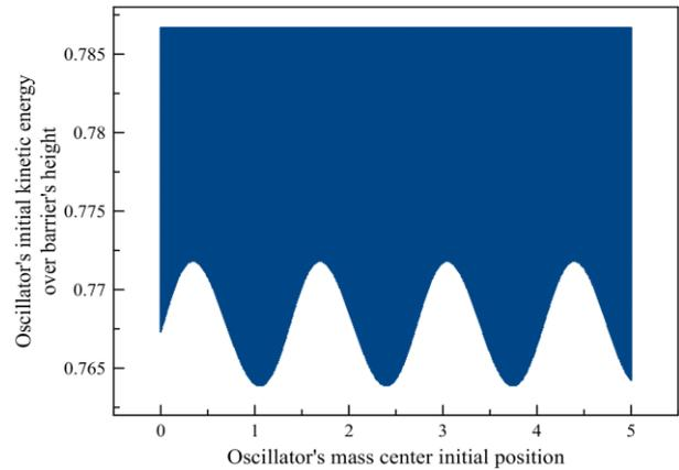
**Figure 1.** Oscillator passes the potential barrier even if its initial kinetic energy is below the barrier's height given the oscillator's length is comparable to the barrier's half-width (blue points show the cases when the oscillator passed the barrier, while white points show the cases of reflection).
