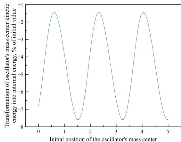
**Figure 3.** Change of oscillator's kinetic energy as a result of transformation into internal energy as a function of initial position of the mass center.
