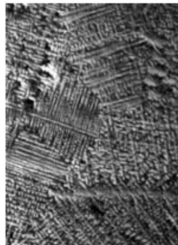
**Figure 6.** Granular structure of material after dendritic crystallization. Notice formation of grain boundaries between dendrites growing with different orientation.
