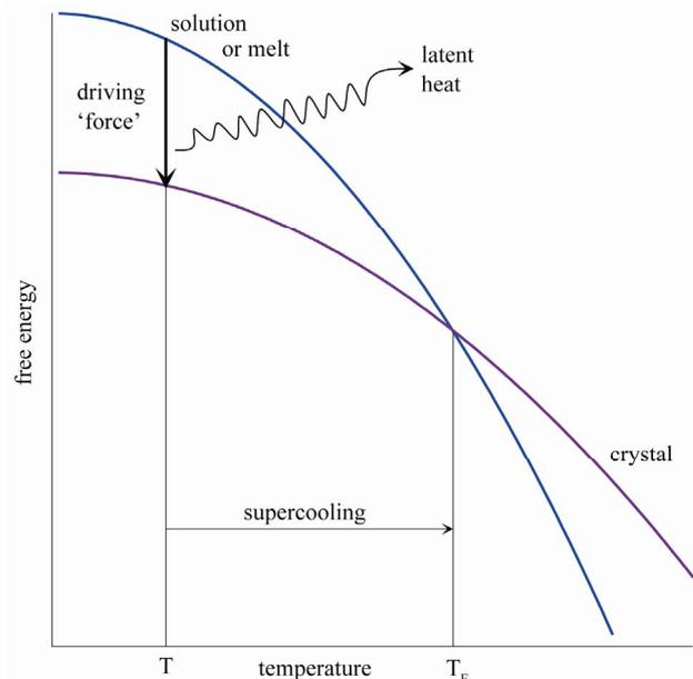
**Figure 2.** Free-energy versus temperature diagram of crystallization.
