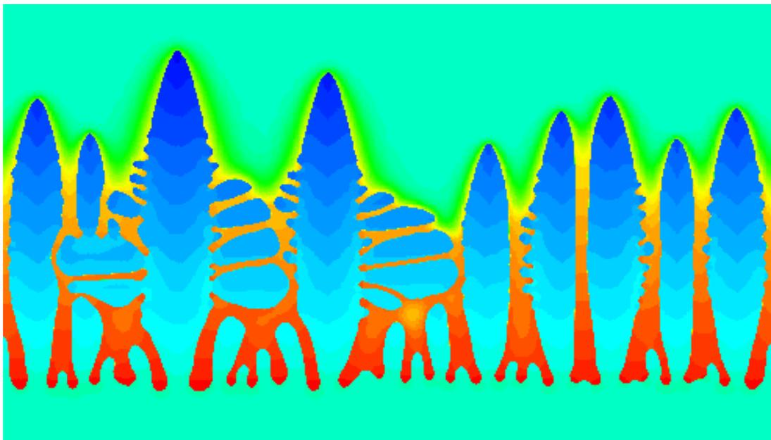
Figure 4. Numerical simulation of the diffusion field between growing crystals during directional solidification. Red, yellow, green, and lime colors represent diffusion field between growing crystals with the red corresponding to the highest concentration (lowest saturation) and lime—to the lowest concentration. (N. Provatas, J. Dantzig and N. Goldenfeld; reproduced with permission).
