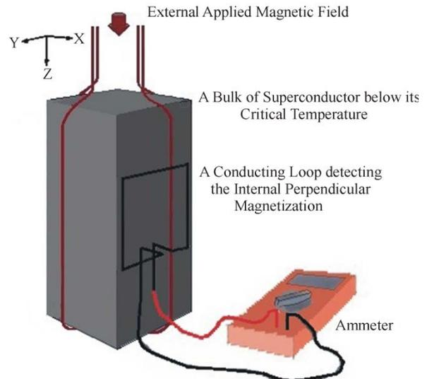
**Figure 2. The Meissner Effect in which an applied external magnetic is expelled by a superconductor. The lines of the external magnetic vector field suggest a magnetization inside the superconductor with the directions perpendicular to the applied external magnetic field (comparing Figure 1(b)).**
