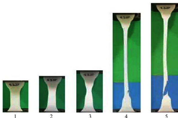
Figure 3. Profile of the plain HDPE sample during characteristic stages of the tensile test.
