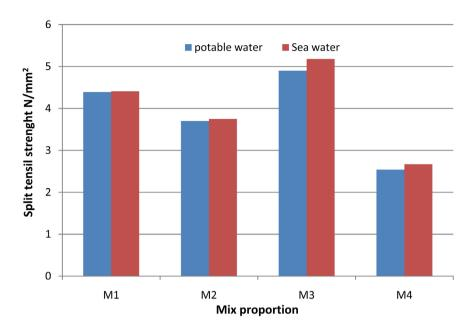
Figure 11. Comparison for split tensile strength with different aggregate in geopolymer concrete.
