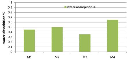
Figure 18. Water absorption of geopolymer concrete with different aggregate.
