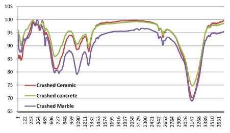
Figure 13. IR spectra of fly ash and slag based geopolymer with different coarse aggregate.
