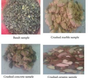
Crushed ceramic sample
