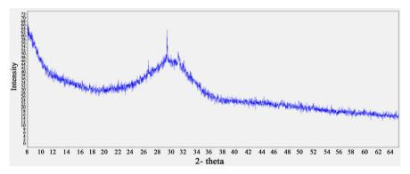
Figure 6. XRD of slag.
