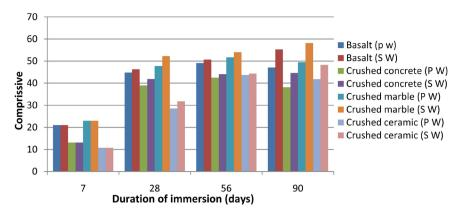
**Figure 10.** Comparison for compressive strength with different aggregate in geopolymer concrete with different water environments.
