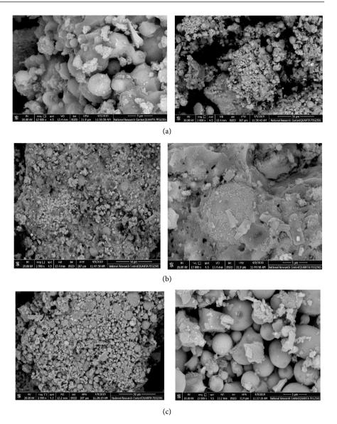
**Figure 12.** SEM-photographs and digital photos of different aggregate of geopolymers. (a) Crushed concrete; (b) Crushed marble; (c) Crushed ceramic.
