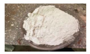
Figure 5. Ground granulated blast furnace slag sample.
