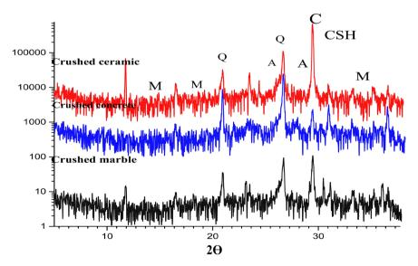
**Figure 14.** XRD patterns for the starting raw material at 28 days (M: Mullite, Q: Quartz, A: Amorphous geopolymer, C: Calcite, C-S-H: Calcium silicate hydrate).
