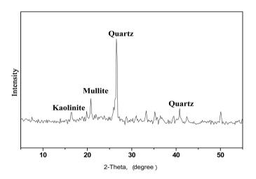
Figure 4. XRD of fly ash.
