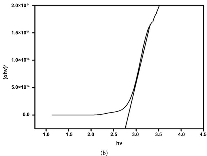
**Figure 4.** (a) Optical transmittance spectrum of 8-HQNB; (b) Plot of  $(\alpha h\nu)^2$  versus photon energy of 8-HQNB.
