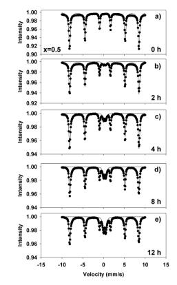
**Figure 10.** Mössbauer spectra of mechanochemically activated  $MoO_2$ -Fe<sub>2</sub>O<sub>3</sub> composites (x = 0.5) at ball milling time of: (a) 0 hour; (b) 2 hours; (c) 4 hours; (d) 8 hours; (e) 12 hours.
