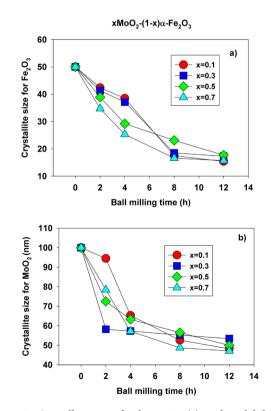
**Figure 7.** Crystallite sizes for hematite (a) and molybdenum dioxide (b) at different molarities and ball milling times.
