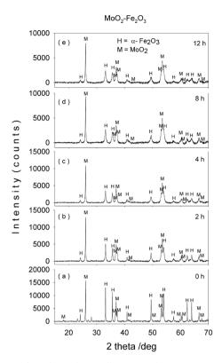
**Figure 3.** XRD patterns of mechanochemically activated  $MoO_2$ -Fe<sub>2</sub>O<sub>3</sub> composites (x = 0.5) at ball milling time of (a) 0 hour; (b) 2 hours; (c) 4 hours; (d) 8 hours; (e) 12 hours.
