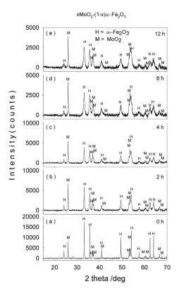
**Figure 2.** XRD patterns of mechanochemically activated  $MoO_2$ -Fe<sub>2</sub>O<sub>3</sub> composites (x = 0.3) at ball milling time of (a) 0 hour; (b) 2 hours; (c) 4 hours; (d) 8 hours; (e) 12 hours.
