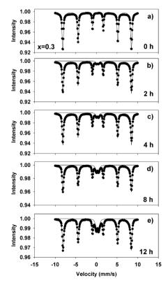
**Figure 9.** Mössbauer spectra of mechanochemically activated  $MoO_2$ -Fe<sub>2</sub>O<sub>3</sub> composites (x = 0.3) at ball milling time of: (a) 0 hour; (b) 2 hours; (c) 4 hours; (d) 8 hours; (e) 12 hours.
