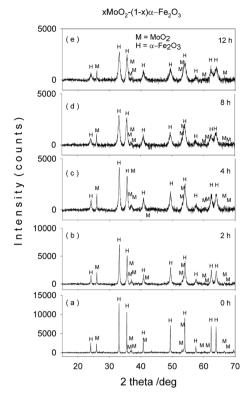
**Figure 1.** XRD patterns of mechanochemically activated  $MoO_2$ -Fe<sub>2</sub>O<sub>3</sub> composites (x = 0.1) at ball milling time of (a) 0 hour; (b) 2 hours; (c) 4 hours; (d) 8 hours; (e) 12 hours.
