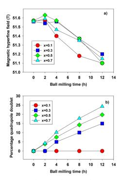
**Figure 12.** Magnetic hyperfine field (a) and percentage of quadrupole doublet (b) as function of molarity and ball milling time.
