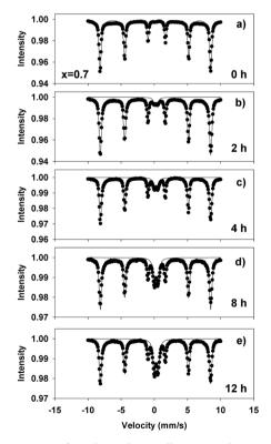
**Figure 11.** Mössbauer spectra of mechanochemically activated  $MoO_2$ -Fe<sub>2</sub>O<sub>3</sub> composites (x = 0.7) at ball milling time of: (a) 0 hour; (b) 2 hours; (c) 4 hours; (d) 8 hours; (e) 12 hours.
