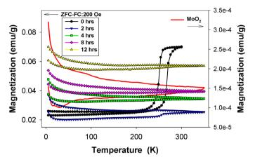
**Figure 15.** Zero-field-cooling-field cooling experiment performed in applied field of 200 Oe between 5 and 300 K.
