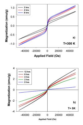
**Figure 14.** (a) Hysteresis loops of the molybdenum dioxide-hematite equimolar system recorded at 300 K in a magnetic field of 5 T. (b) Hysteresis loops of the molybdenum dioxide-hematite equimolar system recorded at 5 K in a magnetic field of 5 T.
