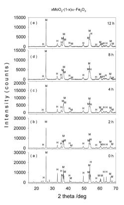
**Figure 4.** XRD patterns of mechanochemically activated  $MoO_2$ -Fe<sub>2</sub>O<sub>3</sub> composites (x = 0.7) at ball milling time of (a) 0 hour; (b) 2 hours; (c) 4 hours; (d) 8 hours; (e) 12 hours.
