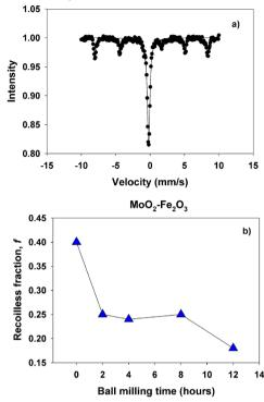
**Figure 13.** Spectrum with stainless steel etalon (a) and recoilless fraction (b) for x = 0.5 and milling time of 0 - 12 hours.
