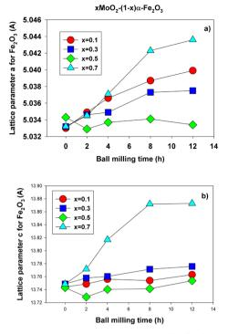
**Figure 5.** Lattice parameters *a* (a) and *c* (b) for hematite at different molarities and ball milling times.
