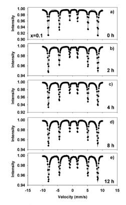
**Figure 8.** Mössbauer spectra of mechanochemically activated  $MoO_2$ -Fe<sub>2</sub>O<sub>3</sub> composites (x = 0.1) at ball milling time of: (a) 0 hour; (b) 2 hours; (c) 4 hours; (d) 8 hours; (e) 12 hours.
