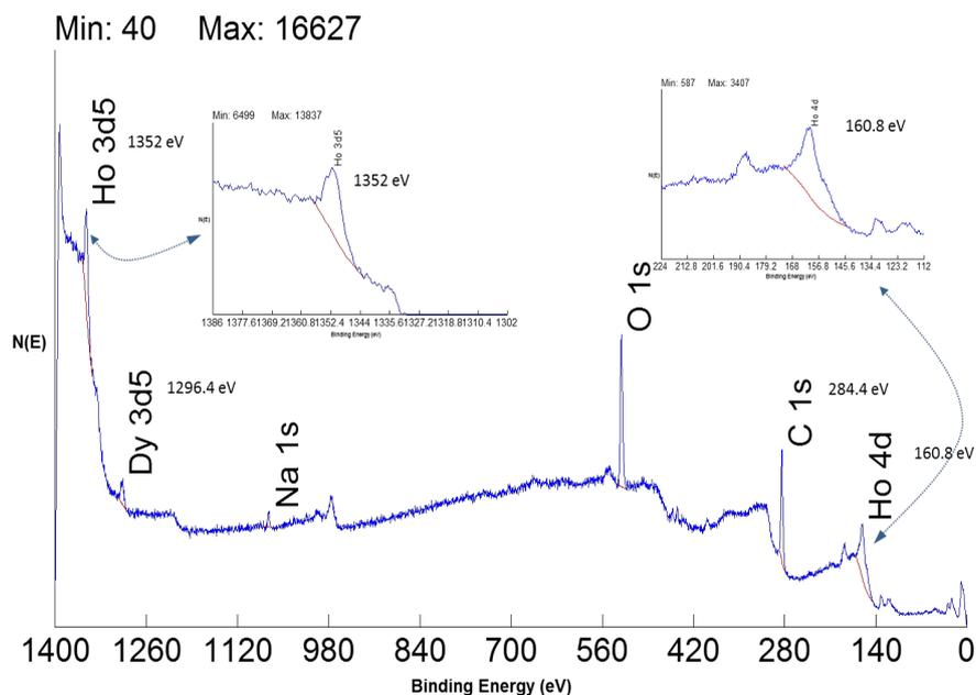
**Figure 6.** XPS spectrum for holmium on polystyrene resin at pH 5.
