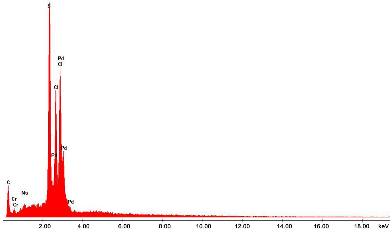
**Figure 9.** EDS of palladium on polystyrene resin.
