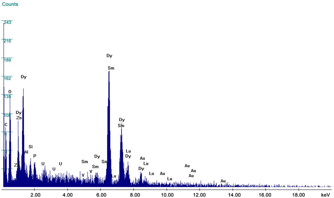
**Figure 2.** EDS of dysprosium on polystyrene/aminophosphonic ion exchange resin at pH 10.
