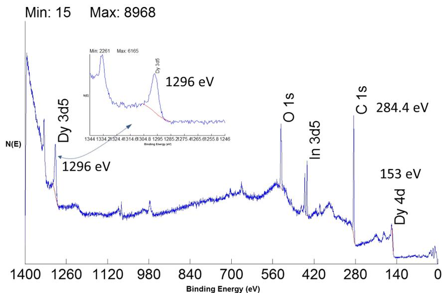
**Figure 5.** XPS spectrum for dysprosium on polystyrene resin at pH 5.
