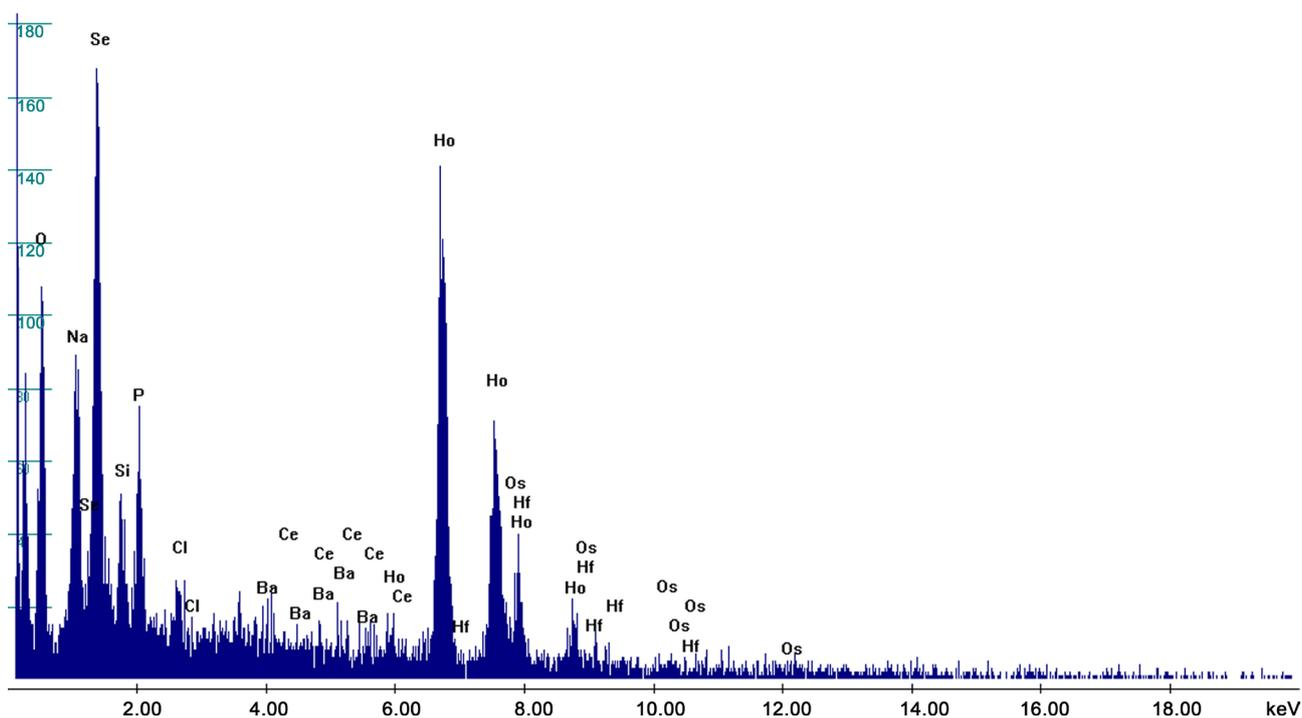
**Figure 4.** EDS of holmium on polystyrene/aminophosphonic ion exchange resin at pH 10.
