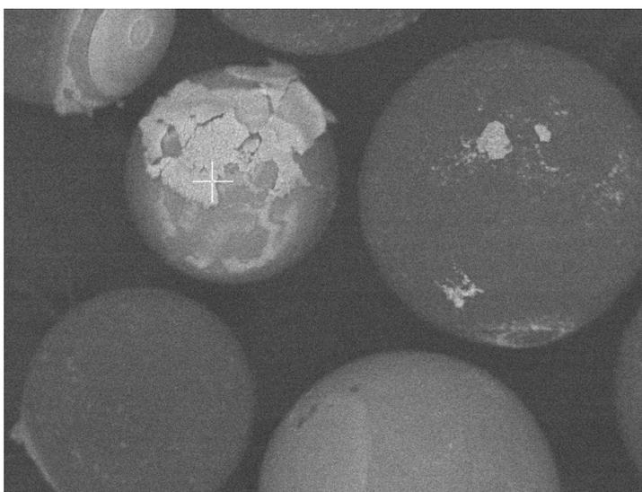
**Figure 1.** SEM of dysprosium on polystyrene/aminophosphonic ion exchange resin at pH 10.
