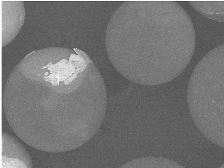
**Figure 3.** SEM of holmium on polystyrene/aminophosphonic ion exchange resin at pH 10.
