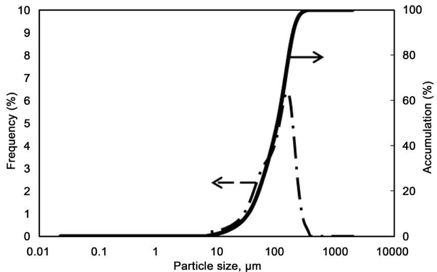
**Figure 2.** Particle size distribution of mine tailing.
