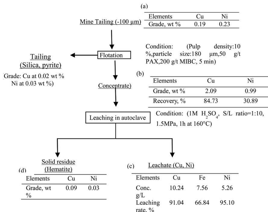
**Figure 13.** Schematic flowsheet for combined flotation and high pressure leaching for recovery of copper and nickel.
