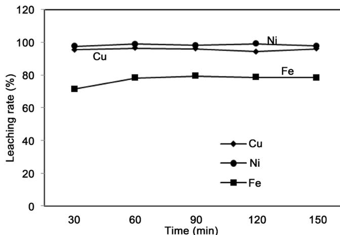
**Figure 11.** Dissolution of copper and nickel from flotation concentrate as a function of leaching time (30 - 150 min leaching, 1 M H<sub>2</sub>SO<sub>4</sub>, S:L = 1:10, 1.5 MPa pressure, 400 rpm stirring speed at 140°C).
