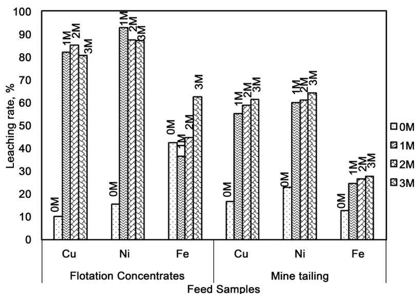
**Figure 8.** Dissolution of flotation concentrate and mine tailing with different concentrations of  $H_2SO_4$  ( $H_2SO_4$ : 0 - 3 M, total pressure 1.5 MPa, S:L = 1:10 at 400 rpm, 140°C temperature for 30 minutes).
