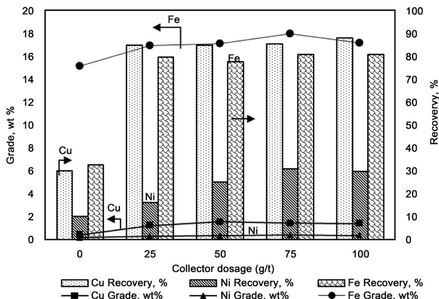
**Figure 4.** Flotation behavior of copper and nickel as a function of collector dosage (Flotation conditions: 10% pulp density, pH 5, and flotation time of 10 minutes).
