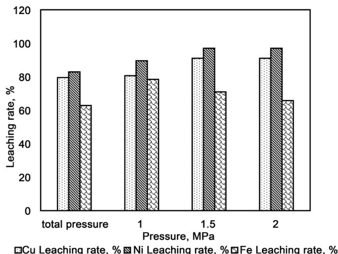
**Figure 10.** Dissolution of copper and nickel from flotation concentrate as a function of pressure (1 M H<sub>2</sub>SO<sub>4</sub>, 1.5 MPa total pressure, S:L = 1:10 at 400 rpm, 140°C temperature for 30 min).
