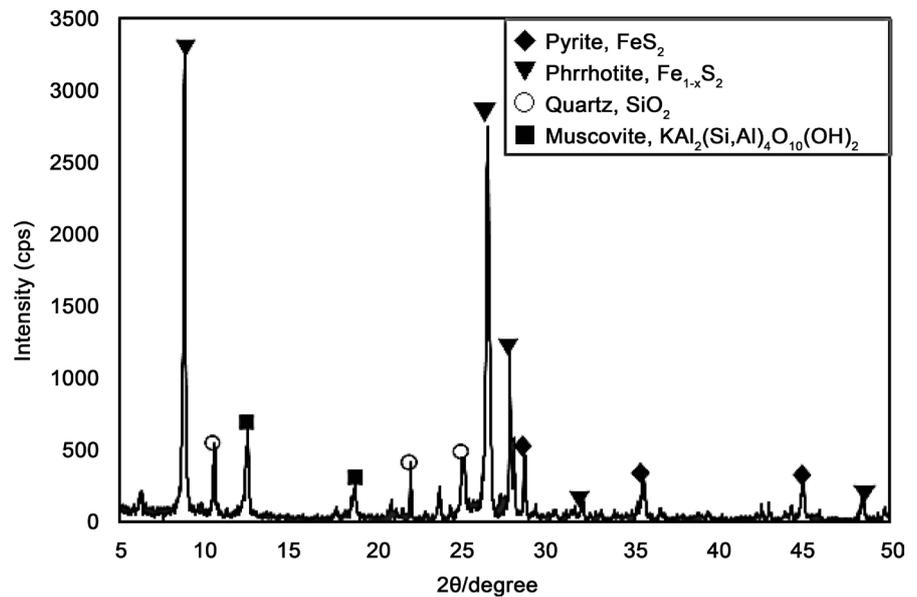
**Figure 1.** XRD pattern of mine tailing.
