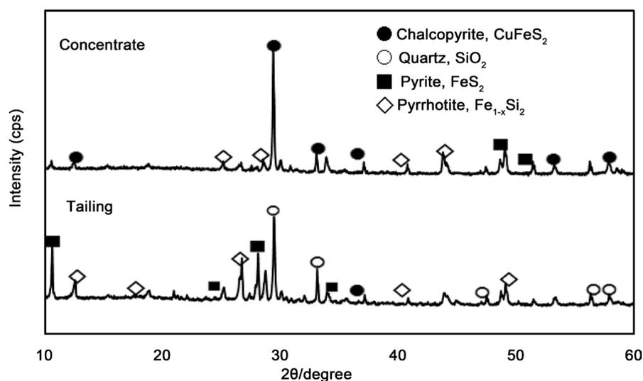
**Figure 7.** XRD patterns of the mine tailing sample and froth concentrate obtained from flotation under the optimum conditions determined (Pulp density: 10%, collector (PAX) dosage: 50 g/t, frother (MIBC) dosage: 200 g/t, at pH 6 for 6 minutes).
