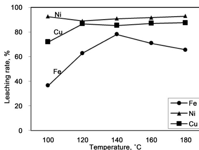
**Figure 9.** Dissolution of flotation concentrate as a function of temperature (1 M H<sub>2</sub>SO<sub>4</sub>, 1.5 MPa total pressure, S:L = 1:10 at 400 rpm for 30 min).
