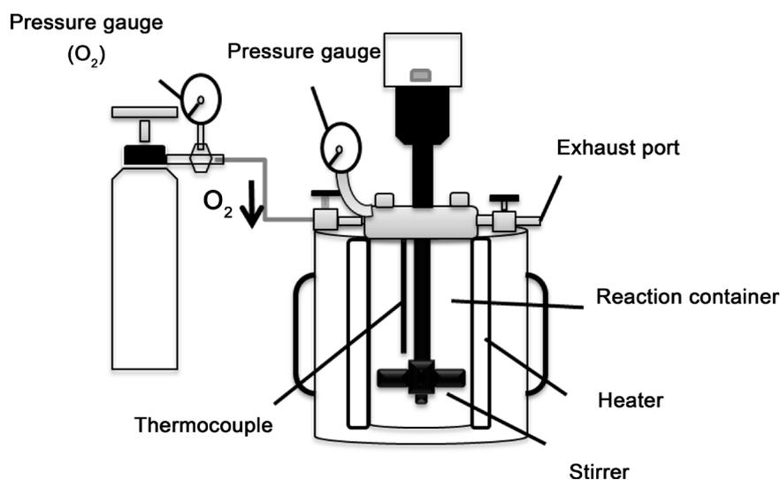
**Figure 3.** A schematic diagram of autoclave equipment used in the study.
