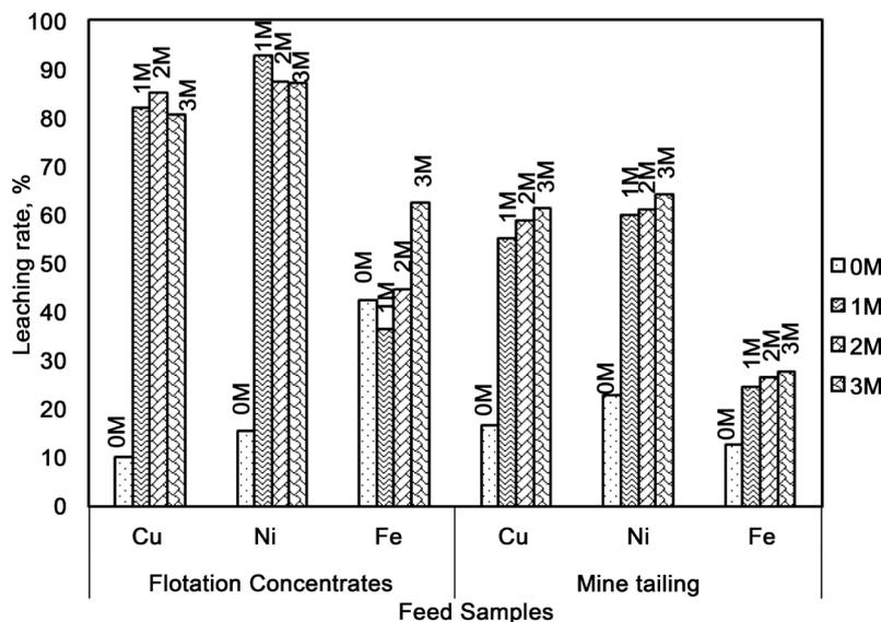
**Figure 8.** Dissolution of flotation concentrate and mine tailing with different concentrations of H<sub>2</sub>SO<sub>4</sub> (H<sub>2</sub>SO<sub>4</sub>: 0 - 3 M, total pressure 1.5 MPa, S:L = 1:10 at 400 rpm, 140°C temperature for 30 minutes).
