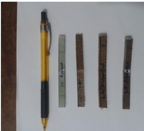
**Figure 7.** Flexural test specimen.
