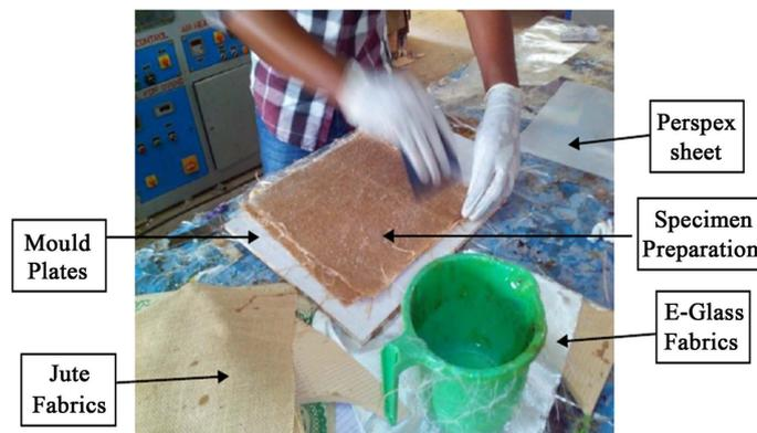
**Figure 1.** Laminates making using hand lay-up technique.
