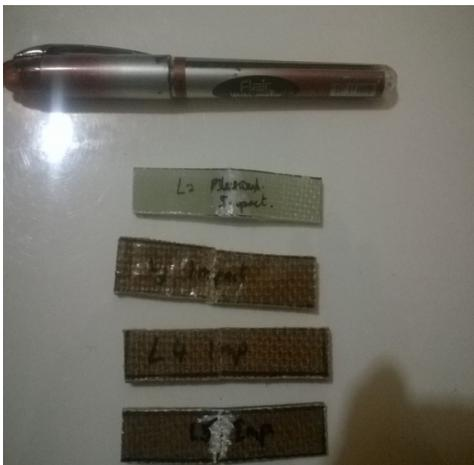
**Figure 8.** Impact test specimen.
