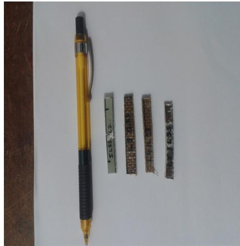
Figure 9. ILSS test specimen.
