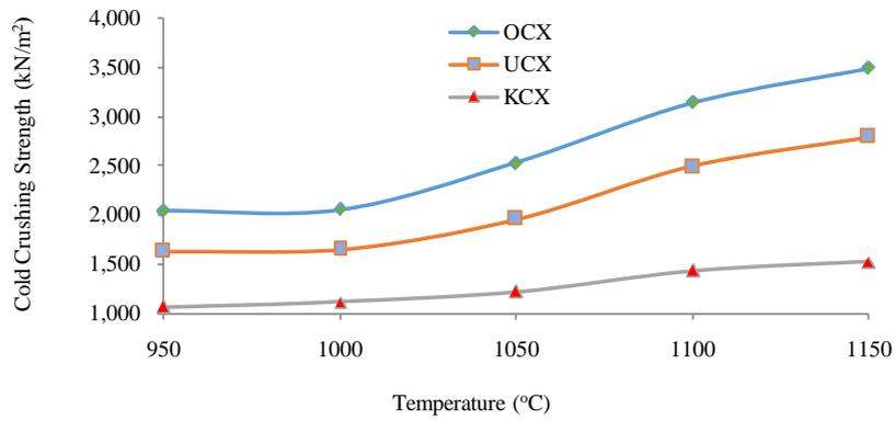
**Figure 10.** Variation of CCS with firing temperature.
