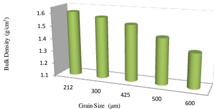
Figure 7. Variation of bulk density of firebricks with grain sizes of wastes.
