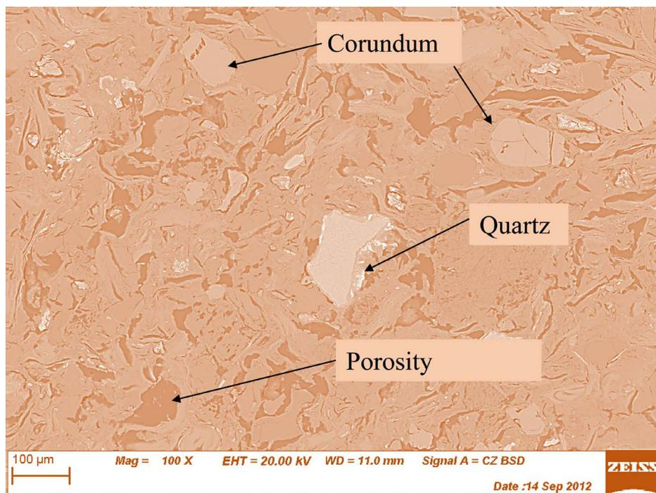
Figure 15. SEM of OTI fired at 1000°C.
