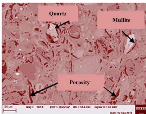
**Figure 5.** Brick without additive fired at 1150°C.
