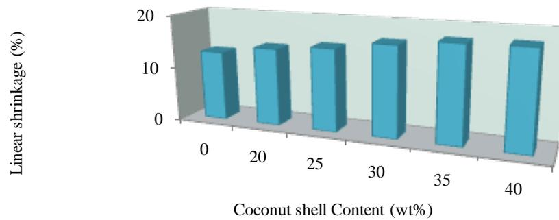
**Figure 3.** Effect of percentage composition of C.S on the linear shrinkage of bricks.
