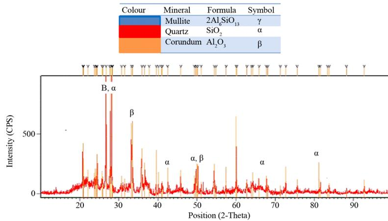
**Figure 11.** XRD of brick fired at 1000°C.
