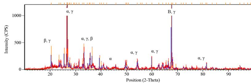
**Figure 13.** XRD of brick fired at 1150°C.
