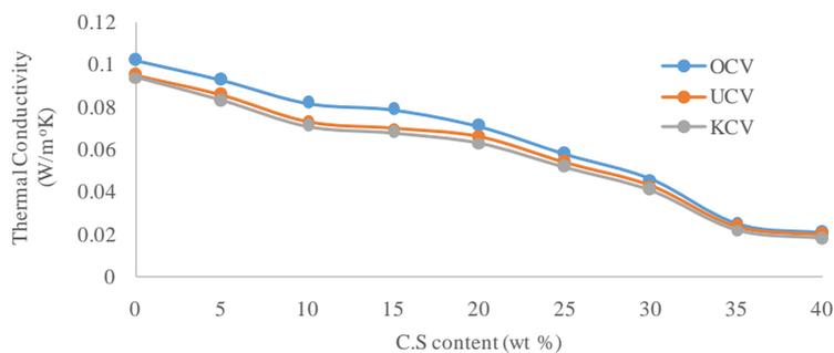
**Figure 4.** Variation of thermal conductivity of the bricks with C.S content.
