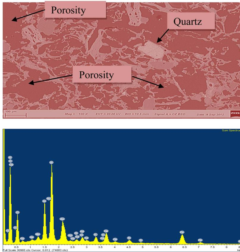
**Figure 1.** EDS and micrograph showing the chemical composition of the brick.
