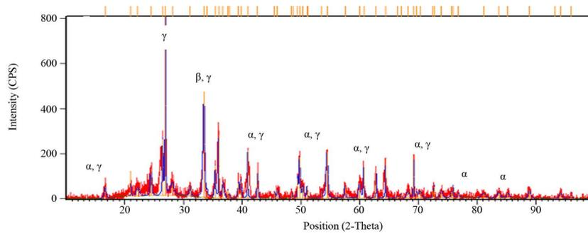
**Figure 12.** XRD of brick fired at 1200°C.
