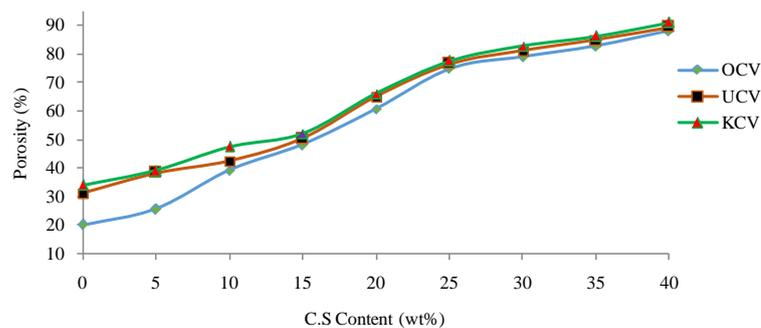
Figure 8. Variation of porosity of bricks with C.S content at 1150°C.
