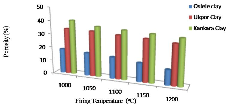
**Figure 9.** Variation of porosity of the brick with the firing temperature.
