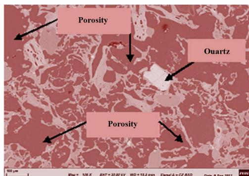
**Figure 6.** Brick with 40% C.S. additive fired at 1150°C.
