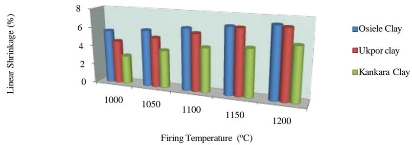
**Figure 2.** Variation of linear shrinkage of bricks produced from various clays at different firing temperatures.
