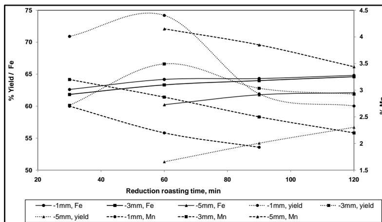
Figure 9. Magnetic separation of the reduction roasting substances.
