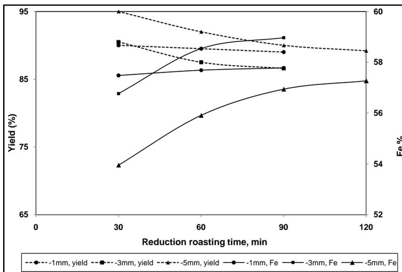
Figure 8. Comparison of reduction roasting products with different feed size at 570°C.
