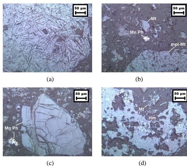
**Figure 10.** Characterization of reduction roasted product. (a): Microplaty magnetite; (b): Mn-phases and microplaty magnetite; (c): Manganiferous phase (pyrolusite) with colloform/botryoidal features; (d): Microplaty magnetite and relict hematite.
