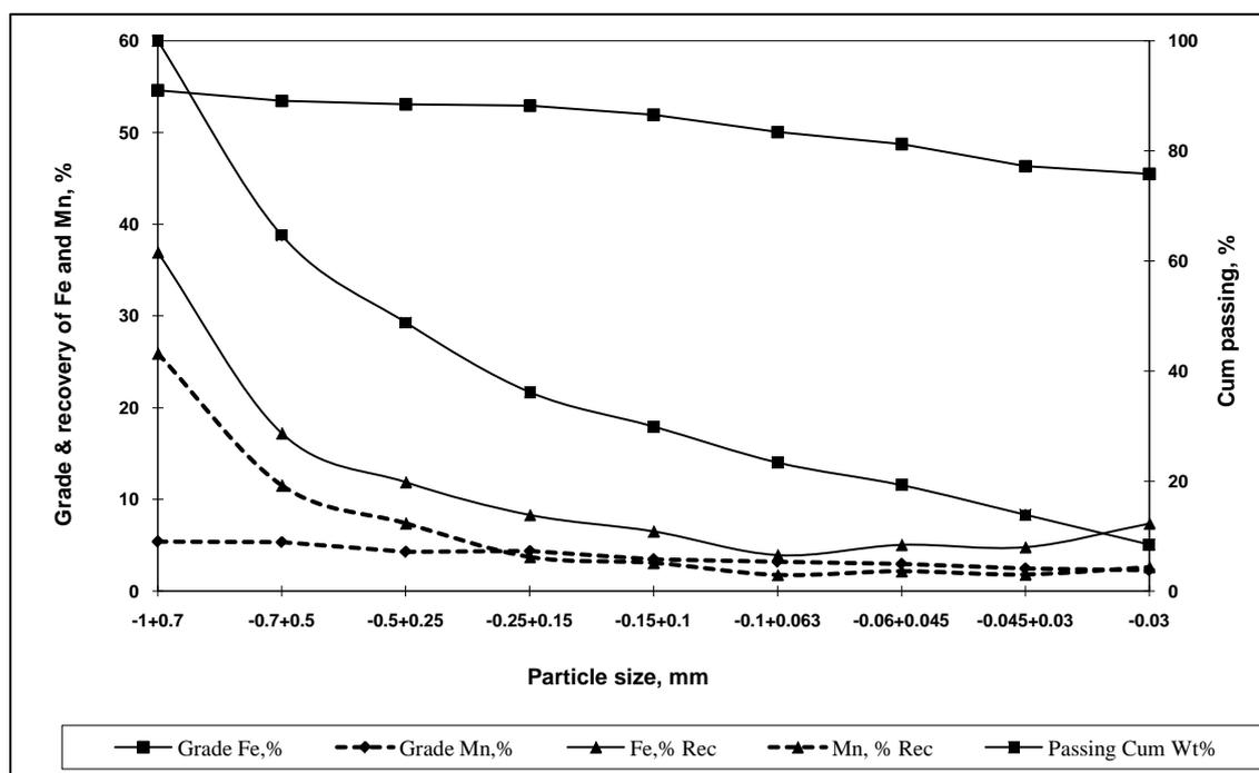
Figure 5. Distribution of particles and their chemistry in crushed to 1 mm.
