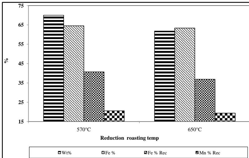
Figure 7. Reduction roasting of -1 mm sample at two different temperatures.
