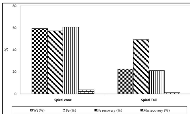
**Figure 6.** Spiralling of hydrocyclone underflow.
