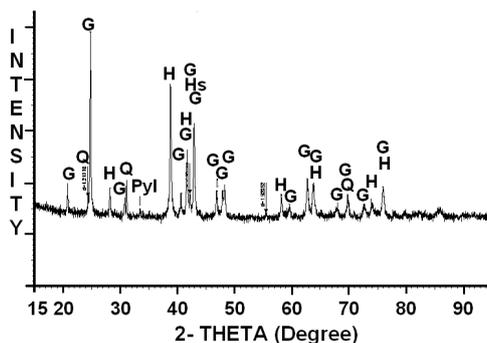
**Figure 4.** XRD of the feed sample. Goethite (G), hematite (H), and magnetite (M) are the major phases. Quartz (Q) and pyrolusite (P) are the minor phases.
