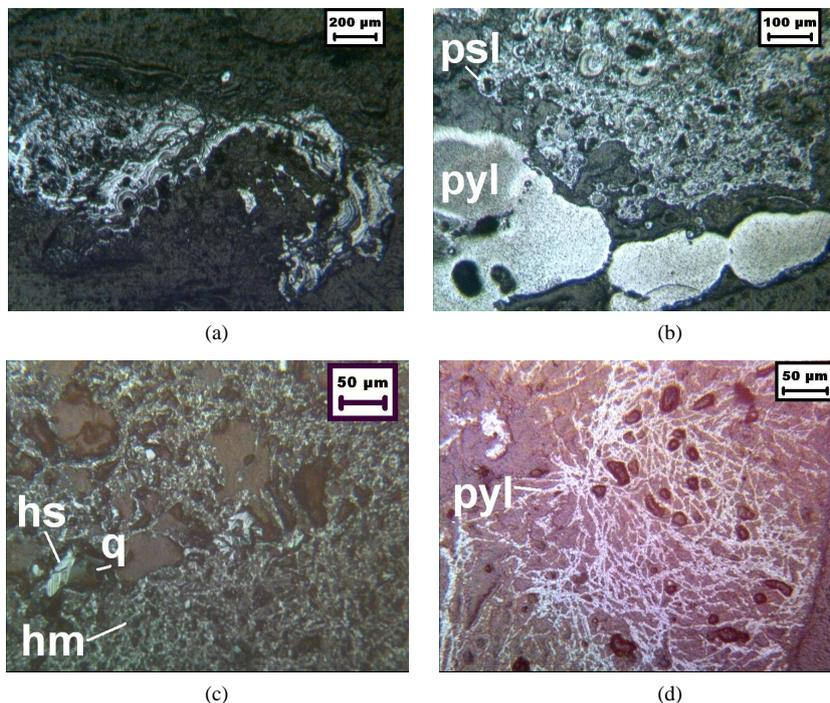
**Figure 3.** Microphotographs of manganiferous iron ore waste fines. (a): Psilomelane; (b): Pyrolusite and psilomelane associated with gangue; (c): Hematite, hausmannite and quartz; (d): Pyrolusite tubes within gangue.
