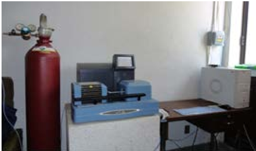
Figure 2. Thermogravimetric analysis equipment SDT600.
