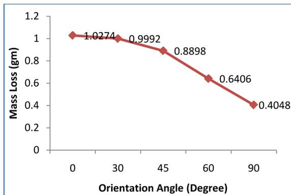
Figure 8. Effect of orientation angle at 10 N.
