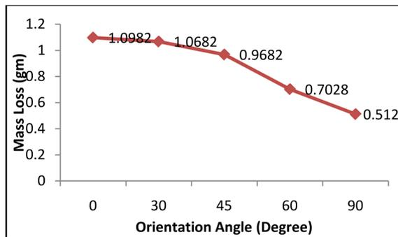
Figure 9. Effect of Orientation angle at 15 N.
