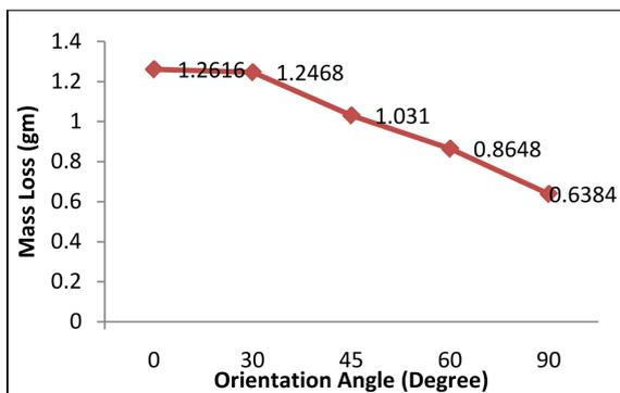
Figure 10. Effect of orientation angle at 20 N.
