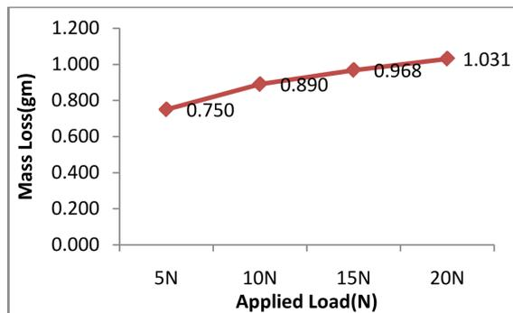
Figure 4. Effect of load at 45° orientation.
