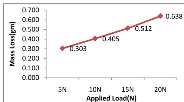
Figure 6. Effect of load at 90° orientation.
