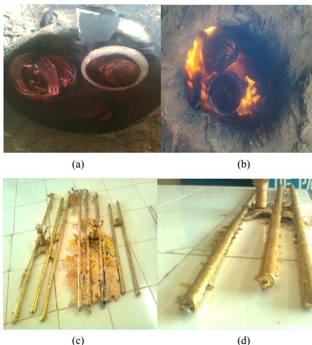
**Figure 1. Charging and cast produced. (a) Charging of copper coils into the pit furnace contained in two crucibles; (b) Ignition of the furnace; (c), (d) aluminium bronze rod cast from the melt. Figures 1(a)-(d) illustrate the production process of aluminium bronze. Pit furnace was used to achieve the melt of charged alloy constituents.**
