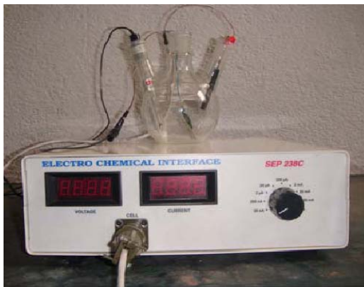
Figure 1. Shows the set up of electrochemical corrosion test rig.
