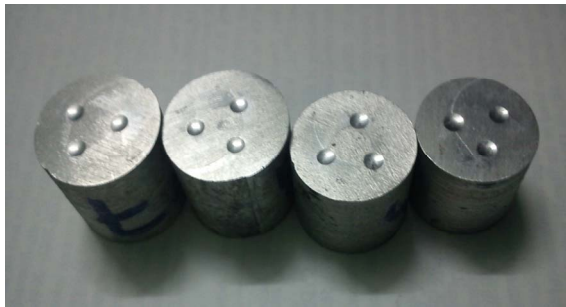
Figure 3. Hardness specimens of Al-5083 composites.
