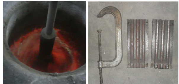
Figure 1. Preparation of Al-5083 composite & CI permanent mould.
