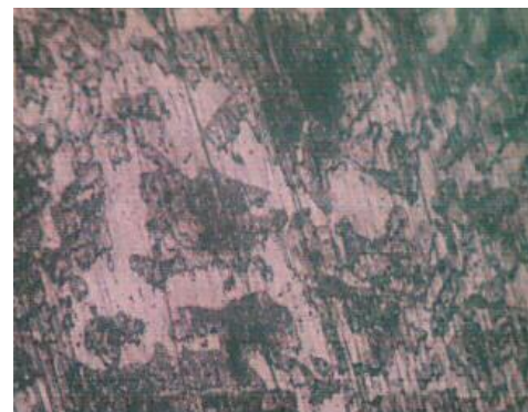
Figure 1. Microstructure of the as-received NST 37-2 steel (400×) (Source: Fadare et al. [24]).
