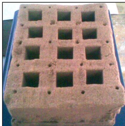
**Figure 1.** Zircon sand mold used to grow Al alloy pieces with different interlayer in O<sub>2</sub> atmosphere.
