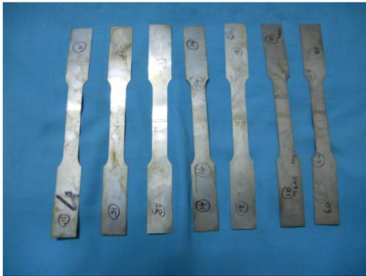
Figure 10. Tensile specimens of inconel 625 welded joints.
