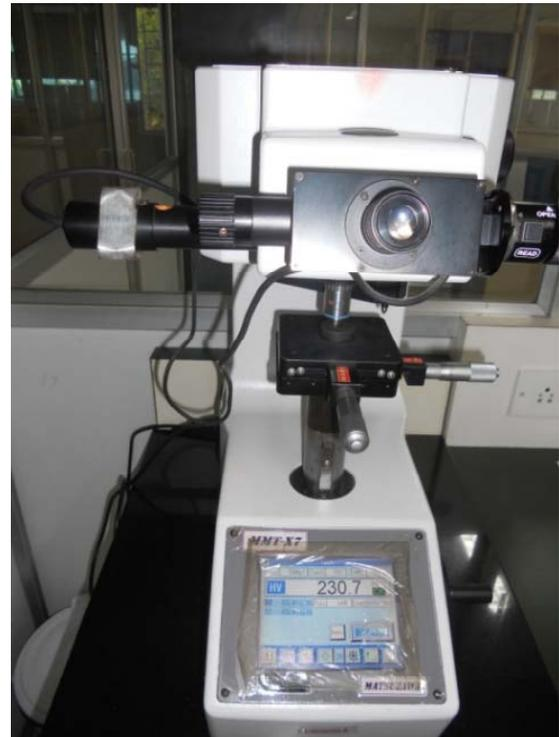
Figure 6. Vickers micro hardness tester.
