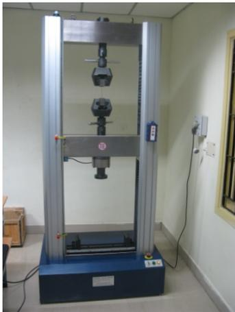
Figure 11. Universal testing machine.
