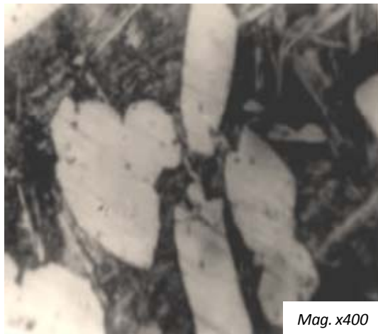
Plate 7. Microstructure of cast Al-Bronze sample subjected to 20% deformation followed by SHT and ageing at 160°C for 6 hours.
