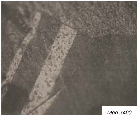
Plate 8. Microstructure of cast Al-Bronze sample subjected to 10% deformation followed by SHT and ageing at 180°C for 6 hours.
