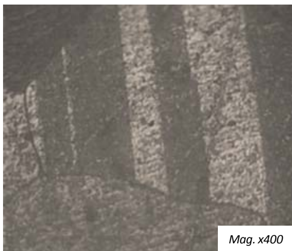
Plate 3. Microstructure of cast Al-Bronze subjected to 20% cold deformation followed by SHT.
