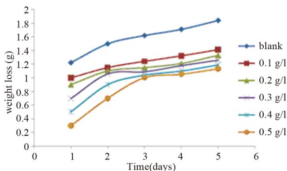
**Figure 1.** Variation of weight loss with different concentrations of *Vernonia amygdalina* extract for the corrosion of mild steel in 0.2 M  $\text{H}_2\text{SO}_4$  at 303 K.
