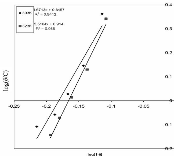
**Figure 4. Flory-Huggins isotherm for adsorption of ethanol extract of *Vernonia amygdalina* on the mild steel surface.**
