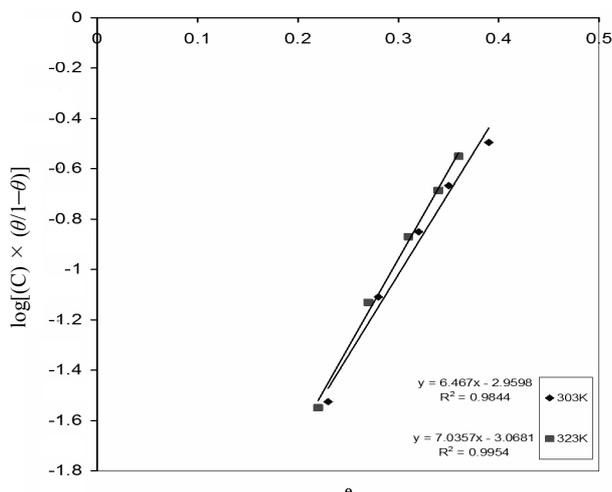
**Figure 5.** Frumkin isotherm for adsorption of ethanol extract of *Vernonia amygdalina* on the mild steel surface.
