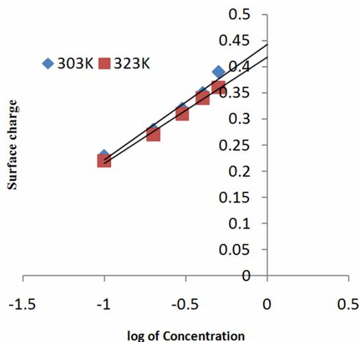
**Figure 3. Temkin isotherm for adsorption of ethanol extract of *Vernonia amygdalina* on the surface of mild steel.**
