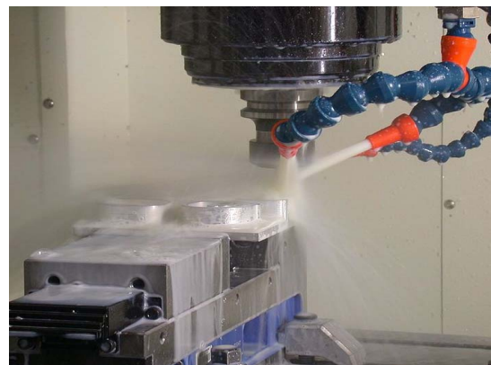
Figure 2. Impulse jet flushing system used.
