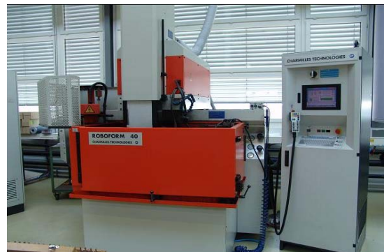
Figure 1. Die-sinking EDM machine used to carry out the experiments.
