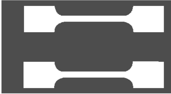
Fig.1 Rolled sheet specimen of powder forged steel having 1 mm thickness With tensile test specimen profiles punched out of it.
