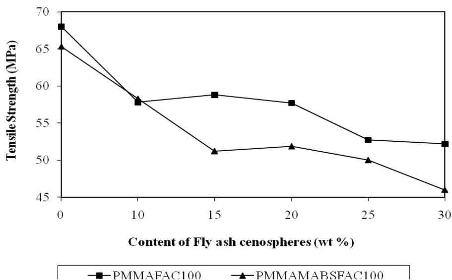
**Figure 1. Variation in Tensile Strength of PMMA/cenospheres (100 mesh) (PMMAFAC100); PMMA/MABS/cenospheres (PMMAMABSFAC100) composites against Content of Fly ash cenospheres (wt%).**
