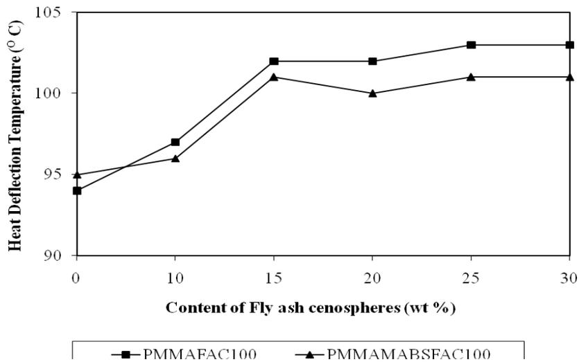
**Figure 7. Variation in Heat Deflection Temperature of PMMA/cenospheres (100 mesh) (PMMAFAC100); PMMA/MABS/cenospheres (PMMAMABSFAC100) composites against Content of Cenospheres (wt%).**
