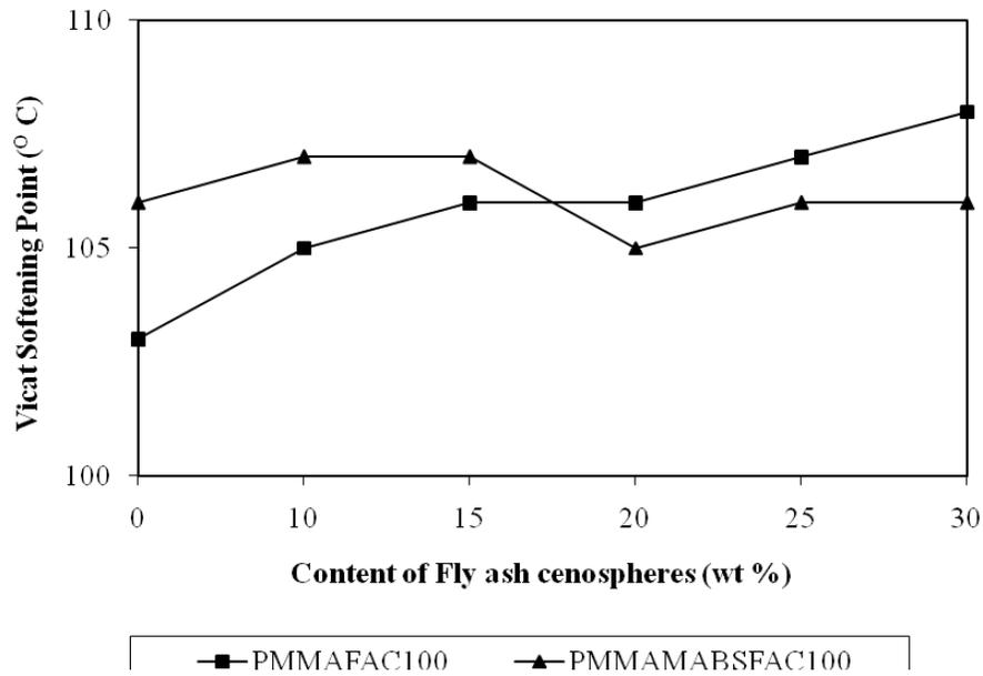
**Figure 6. Variation in Vicat Softening Point of PMMA/cenospheres (100 mesh) (PMMAFAC100); PMMA/MABS/cenospheres (PMMAMABSFAC100) composites against Content of Cenospheres (wt%).**
