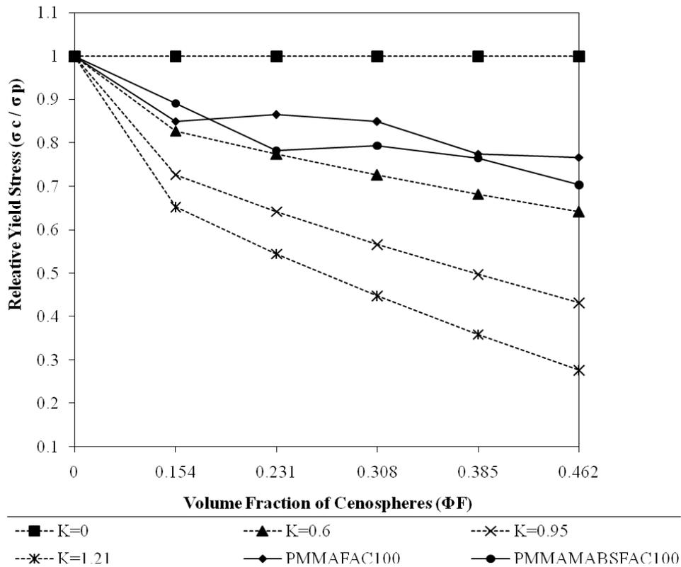
**Figure 3. Variation in Relative Yield Stress ( $\sigma_c / \sigma_p$ ) of PMMA/cenospheres (100 mesh) (PMMAFAC100); PMMA/MABS/cenospheres (PMMAMABSFAC100) composites against Volume Fraction of Cenospheres ( $\Phi F$ ).**
