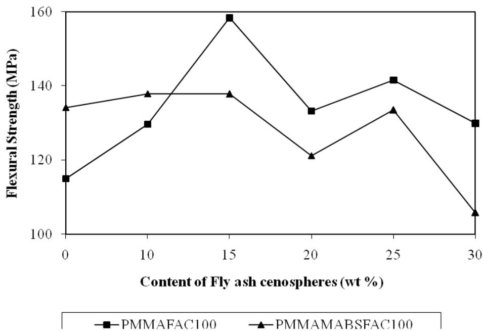
**Figure 5. Variation in Flexural Strength of PMMA/cenospheres (100 mesh) (PMMAFAC100); PMMA/MABS/cenospheres (PMMAMABSFAC100) composites against Content of Cenospheres (wt%).**
