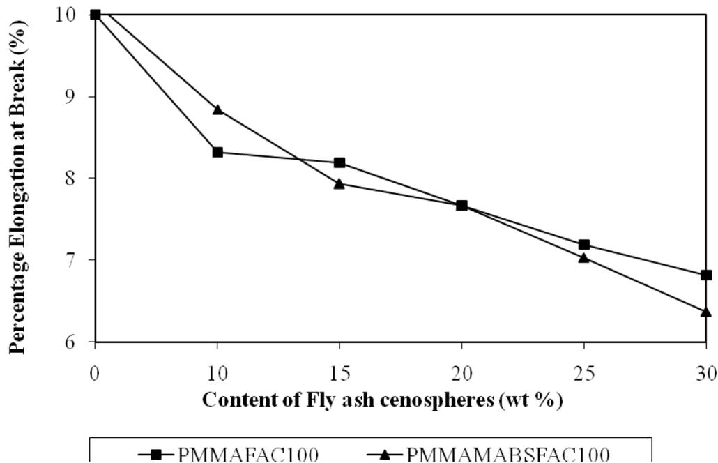
**Figure 2. Variation in Percentage Elongation at Break of PMMA/cenospheres (100 mesh) (PMMAFAC100); PMMA/MABS/cenospheres (PMMAMABSFAC100) composites against Content of Fly ash cenospheres (wt%).**
