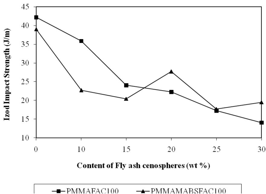
**Figure 4. Variation in Izod Impact Strength of PMMA/cenospheres (100 mesh) (PMMAFAC100); PMMA/MABS/cenospheres (PMMAMABSFAC100) composites against Content of Cenospheres (wt%).**
