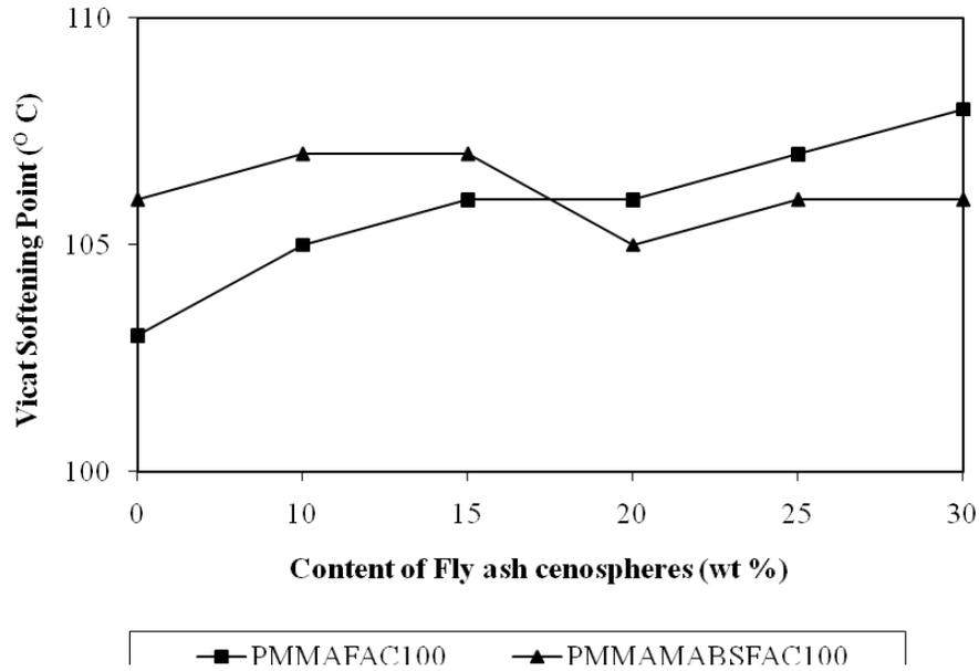
**Figure 6. Variation in Vicat Softening Point of PMMA/cenospheres (100 mesh) (PMMAFAC100); PMMA/MABS/cenospheres (PMMAMABSFAC100) composites against Content of Cenospheres (wt%).**
