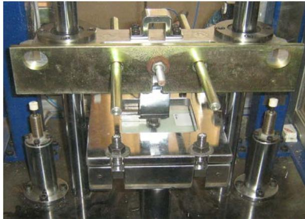
Figure 5 Specimen clamping apparatus
