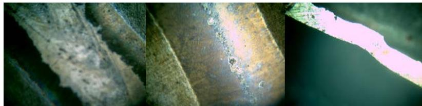
Fig.3 Macrographs of weld pool at 100X
