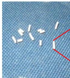
**Fig. 9 (a). Small fillers for *in vivo* testing**
