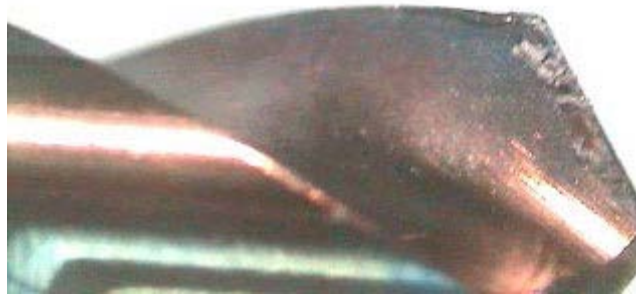
Figure 1 Chip adhered on the cutting lip of the coated drill after the 10th drilling hole
