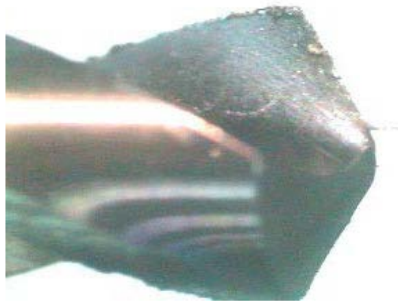
Figure 2 Chip adhered on the cutting lip of the coated drill after the 12th drilling hole
