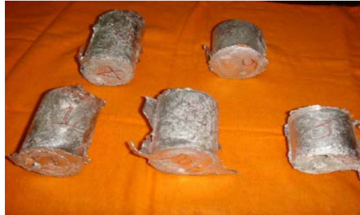
Fig.2 : Hybrid aluminium metal matrix composite (Al6061-SiC-Al 2 O 3 ) at different wt.%
