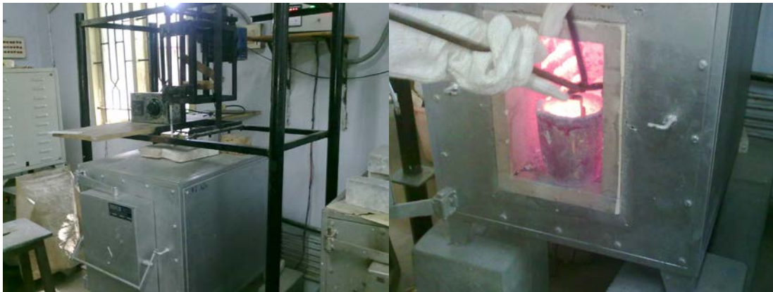
Fig.3 The experimental set up used in fabrication of hybrid MMC (Al6061-SiC-Al 2 O 3 ) composites
