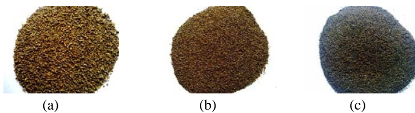
Plate 2.2 Ore Sample Particle Size Fractions (a) 1.00/0.50mm, (b) 0.50/0.25mm, (c) 0.25/0.125mm
