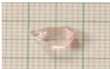
Fig. 4. Molybdenum doped KTP crystal grown from KTP/Flux ratio 7:3. ( 7 \times 5 \times 2.5 mm 3 ).
