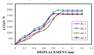
Figure 10. Load Vs displacement plot along the fiber direction
