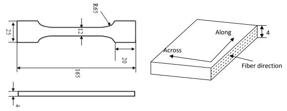
Figure 1. Specimen prepared directions with fiber directions
