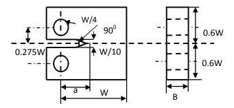
Figure 2. Standard specimen dimensions
