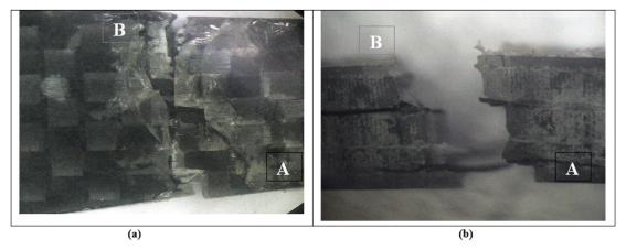
Figure 8. Glass-Carbon epoxy hybrid composite test coupon after tensile test showing (a) front view and (b) side view. With a magnification of 4X
