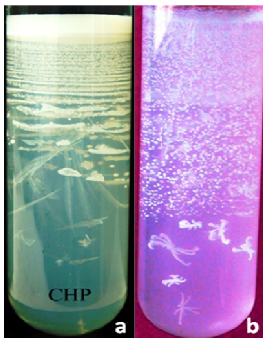
Fig. 1. Calcium phosphate crystals in the test tubes (a) pure (b) 0.2M \text{SrCl}_2 added
