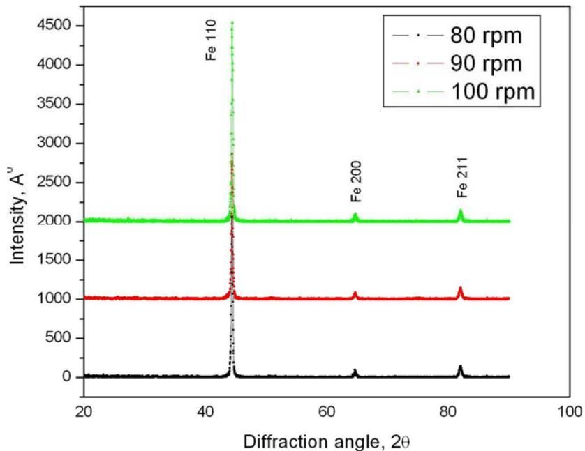
**Fig.2 XRD pattern of machined chip of AISI 304 SS at different cutting speed**
