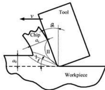
**Fig.3 Schematic of plane strain machining with other parameters**
