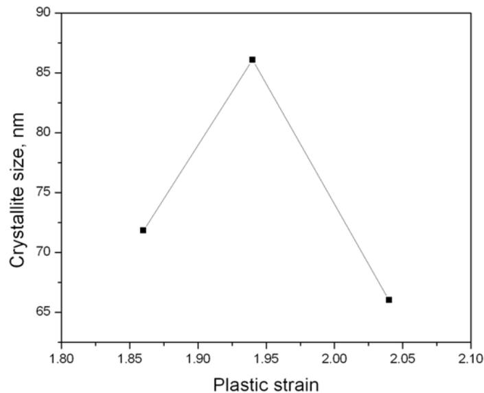
**Fig. 4 (a) Effect of plastic strain on crystallite size**
