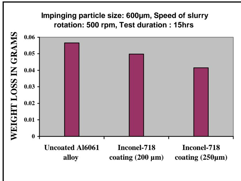
**Fig. 5: Effect of coating thickness on slurry wear loss at slurry concentration of 100 g/litre**
