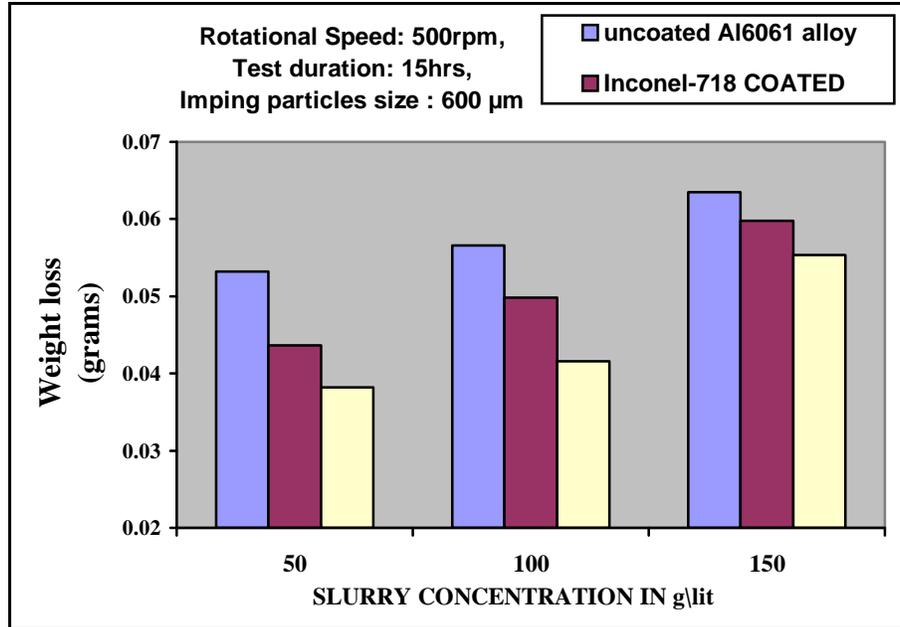
**Fig.4 Effect of slurry concentration on slurry erosive wear of Inconel-718 coatings**
