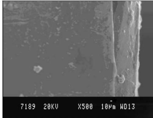
**Fig. 2 SEM of cross sectional micrograph of Inconel-718 on Al6061 alloy**
