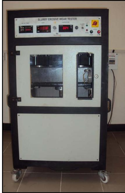
**Fig. 1 Photograph of slurry erosion wear tester**
