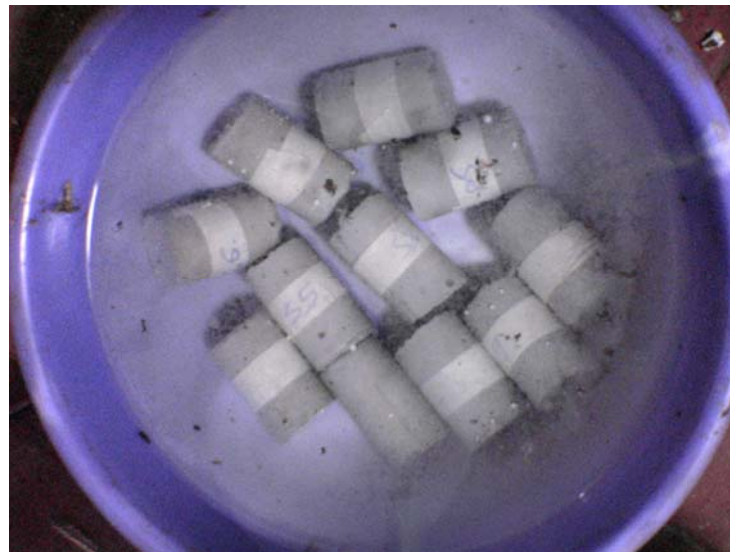
Fig.3: Cured Brick Samples
