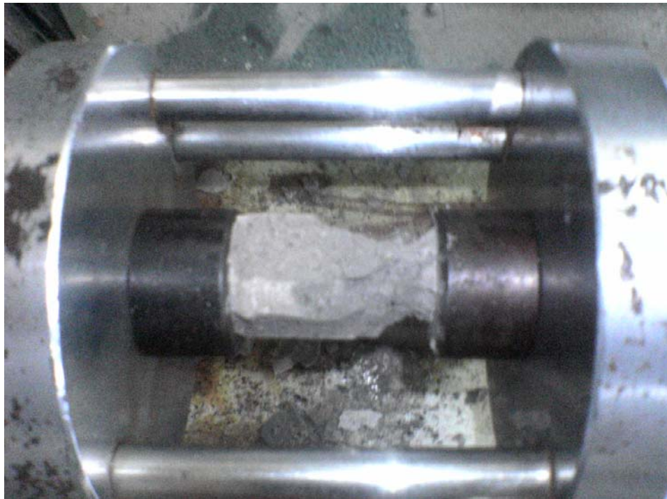
Fig.4: Brick fracturing during compression
