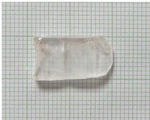
Fig. 2. As grown LGAHCB single crystal
