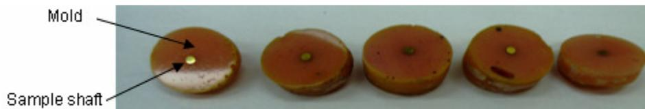
Fig. 2 Sample prepared for polishing and etching
