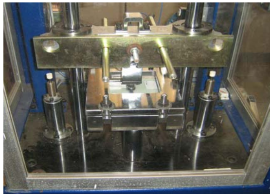
Figure 2. Specimen clamping apparatus
