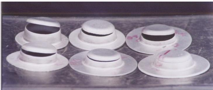
Fig. 1: Broken cups using 64, 65 and 70/33mm draw ratios
