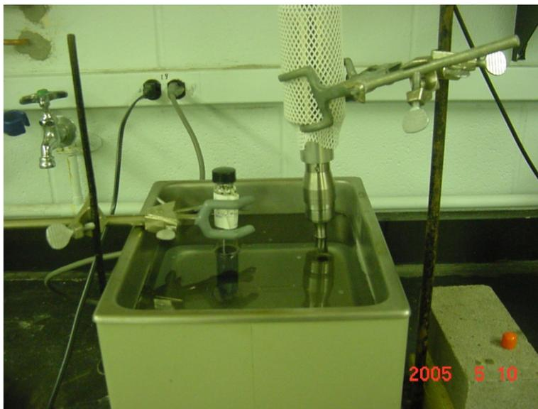
**Figure 1.** Typical double sonication system used in dispersing SWNT. The system consists of an ultrasonic bath and an ultrasonic probe on the right.
