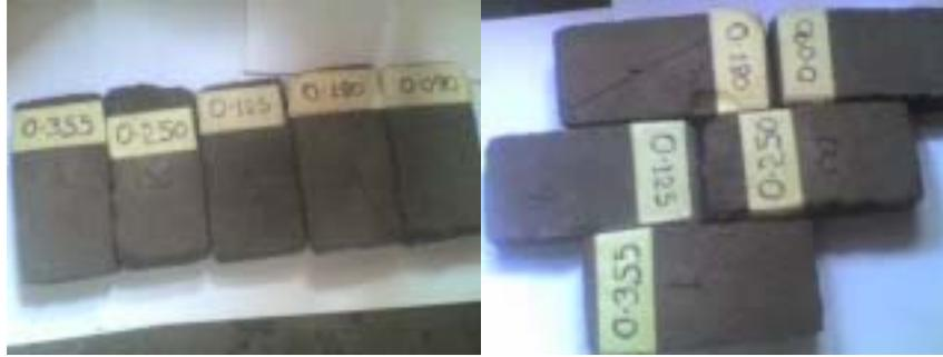
Plate 2. Photo of the produced bricks after firing.
